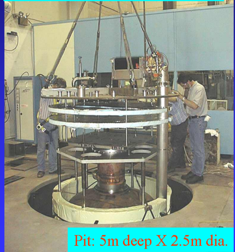
Cavity going into test pit in Newman basement
