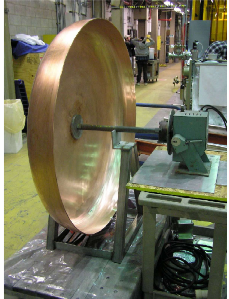
Mechanical cleaning of the cavity inner surface (right) after e-beam welding of the stiffener ring (above)
