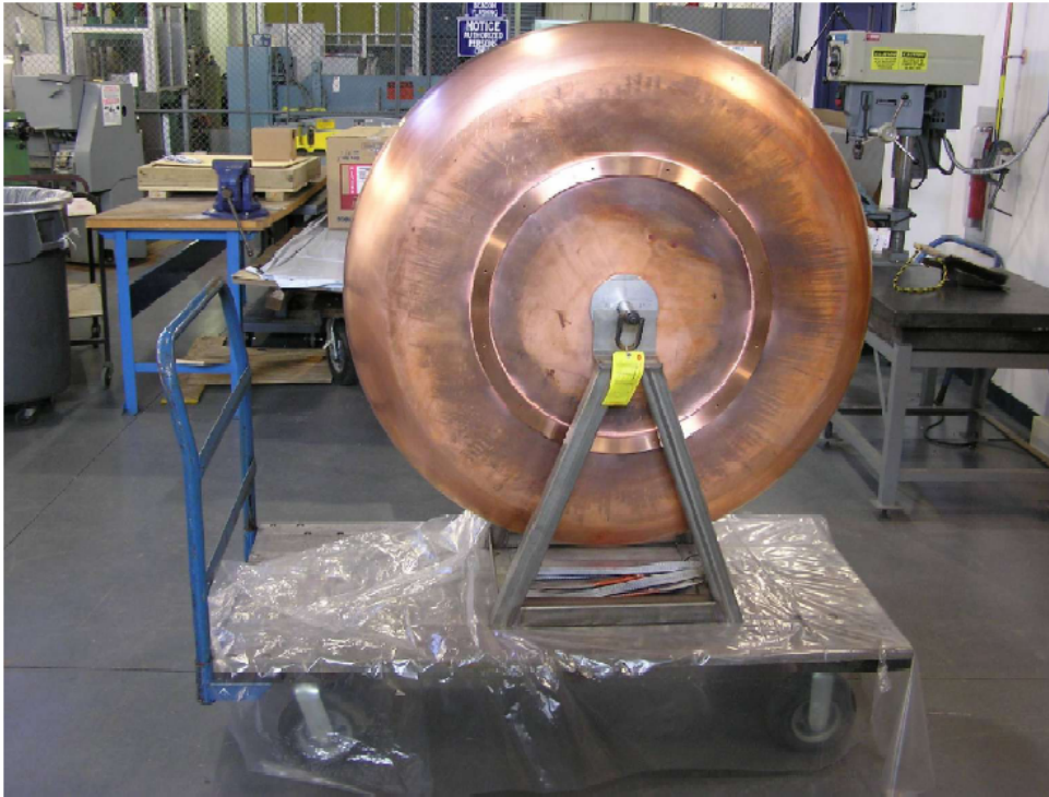
Mechanical cleaning of the cavity inner surface (right) after e-beam welding of the stiffener ring (above)
