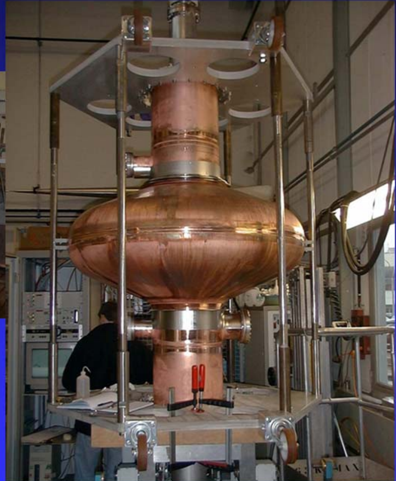
Magnetron Nb film (1-2 \mu\text{m} ) sputtering
