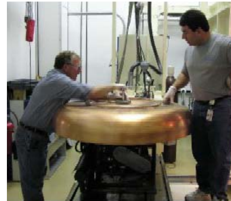
201 MHz half-shell ebeam welding of Stiffening – JLab
