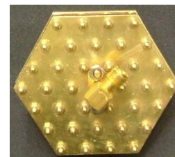
Figure 2: A photo of the realized PBG; it is shown a connector used to excite and to measure the field inside the structure.
