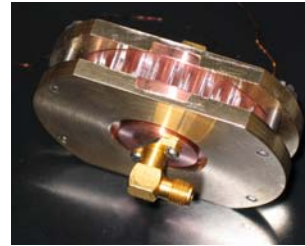
Figure 5: The hybrid PBG: dielectric cylinders on copper plates. Here it is shown a connector and the external clamping system.
