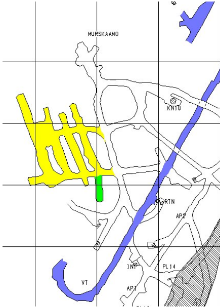
Figure 2. Schematic view of the caverns at 660 metres underground. The yellow-coloured areas (at the left) can be used for the scientific purposes. These include an old lunch room (green), and many service and storage rooms, largest of them is of the size of 30\text{ m} \times 10\text{ m} \times 8\text{ m} . The blue-coloured area in the middle is the spiral-shaped decline, and the shadowed area in the right-lower corner shows the mining zone.
