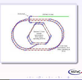
C.R. Prior MW Proton Drivers using Rapid Cycling Synchrotrons
